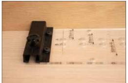
Place the acrylic jig template on top of your mark and line up to the center of the pre-drilled hole. Make sure that you are using the appropriate side of the template for your setback. In this example we are working this project using the 37mm setback, so that edge is up against the corner of the cabinet.
