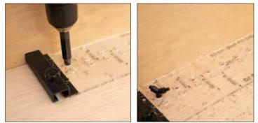
Drill the first hole at the bottom of the jig with the appropriate drill bit (either ¼" or 5mm drill bit – both are included). Once the hole is drilled. DO NOT drill anymore holes until you continue to the next step
