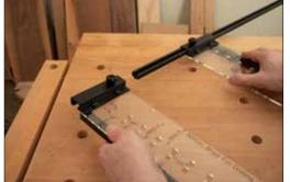
Loosen the studded round knob at the top and bottom of the jig templates. If installed, remove the M4x3/16" Socket Head Stop Screws and Washers (Parts 1 & 2). Slide the jigs off of the long track rails.
