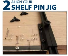
With the shelf pin jig fully assembled, place the jig onto your stock and close both sides of the jig up against the sides of your stock piece. Lock the jig by securing each of the round knobs securely. Align the jig with the first hole on the bottom of the jig as shown here. Make sure both sides of the jig properly align with the marks made in the previous step.
