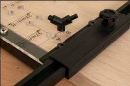
Insert the star shaped indexing pin. The indexing pin has two different dowel tips. One is <sup>1</sup>/<sub>4</sub>" in diameter and the other is 5mm in diameter. Use the appropriate pin size for the holes you just drilled. Make sure the pin is full seated into the hole before proceeding.
