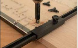
Drill the first hole at the bottom of the jig with the appropriate drill bit (either  $\frac{1}{4}$ " or 5mm drill bit – both are included). Once the hole is drilled. DO NOT drill anymore holes until you continue to the next step
